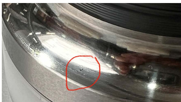
Surface contamination on the ball raceway of a wheel bearing inner ring in overview and close-up, along with the corresponding C-image from the Eddyvisor test instrument after completion of the inspection. @ibg
