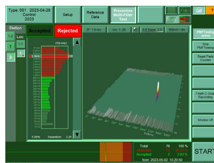
Surface contamination on the ball raceway of a wheel bearing inner ring in overview and close-up, along with the corresponding C-image from the Eddyvisor test instrument after completion of the inspection. @ibg
